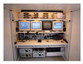
Electronic map shows the locations of the rescue teams equipped with radio devices. Professional analogue mobile radio devices (PAMR) are used. They are able to send the GPS position to the vehicle command center.
