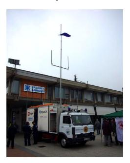
The vehicle's is heavily equipped with radio communication devices. Coordination of teams in disastrous events is mostly executed by radio communications. Tall antenna ensures the vehicle the larger area of coverage for radio devices of the teams under control.
